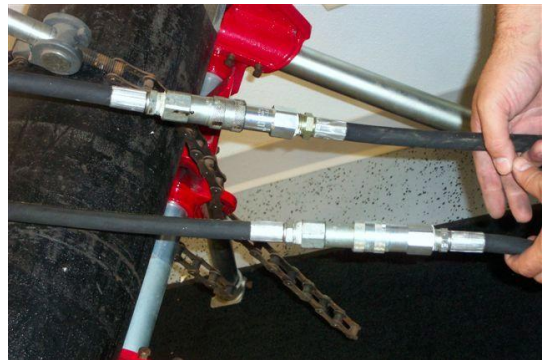
Lines attached to PipeMaster
