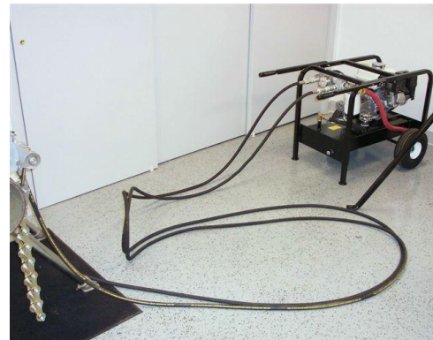
Lines attached to the Power Pack
